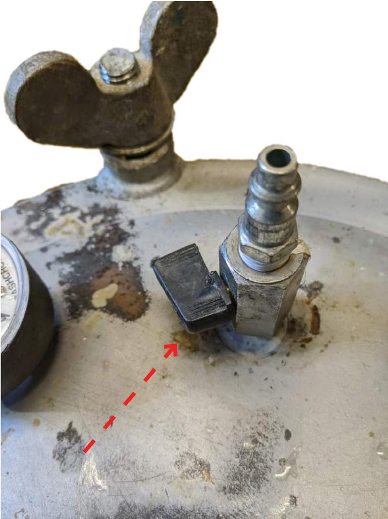
After the hose is connected, turn the black lever slowly until it is parallel with the hose.
