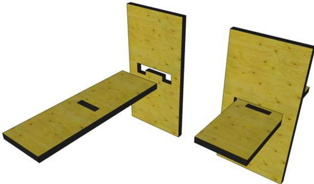
Such joints may be useful especially for shelves or other upright applications where gravity can be exploited to keep the pieces engaged, and may be biased or otherwise modified like the "T" joints described below.
