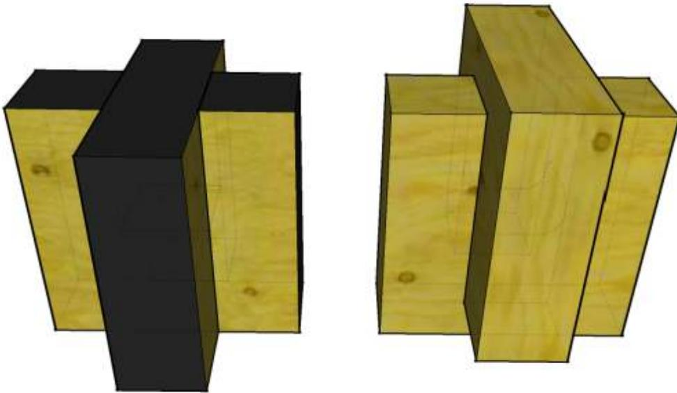
The router-cut version, however, doesn't work. The radiused corners bump into each other and the part edges don't line up. You can cut each slot a bit deeper, of course, and in some applications this may be OK, but doing so leaves a void in the center of the joint and concentrates stress on the radiused corners. A better solution is this:
