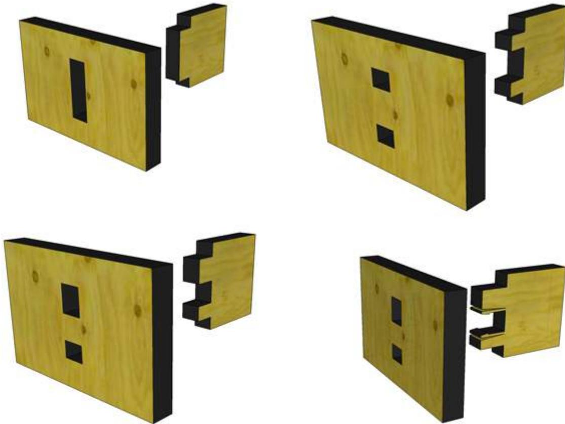
Here is a simple "mortise and tenon" type joint. We can split the "mortise" and "tenon" into two slots and tabs (or into as many slots and tabs as we like). If we break the symmetry of the slots and tabs, the joint becomes biased. And if we extend the tab a small distance past the thickness of the stock, we can easily add snaps or detents that catch on the far side of the slotted part.
