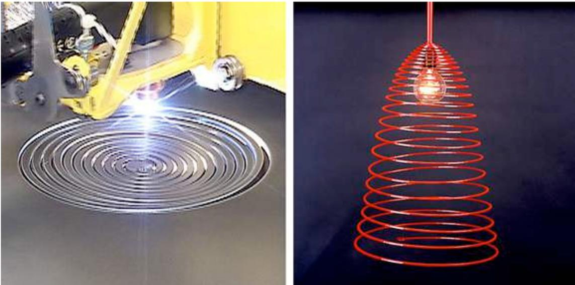
Finally, here's an oddball free-hanging spiral technique, courtesy of the good folks at PlasmaCAM. The spiral is cut out of a piece of steel using a CNC plasma cutter, but the same idea could work with a laser cutter or a mill, in a different material.
