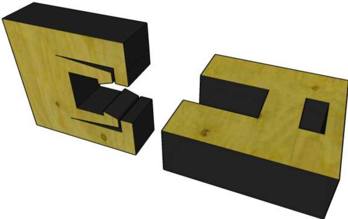
But move the hook and the catch away from the edges of the stock, and the snap-lock action becomes "irreversible." Note that both pieces of stock could include both hooks and catches. I'm only showing "one sided" snapping joints for clarity.
