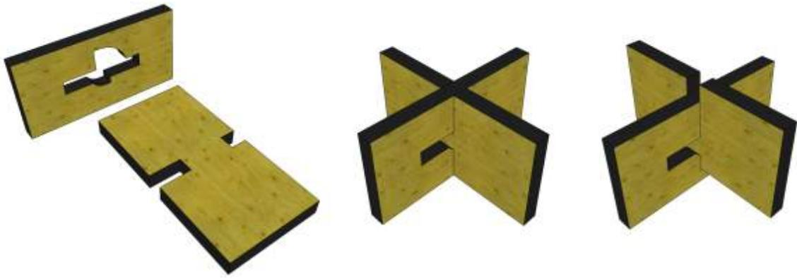
A biased version is also possible. Here's a similar joint with the symmetry broken shown disassembled (left), assembled in favored orientation (middle), and assembled in its "disfavored" orientation (right).
