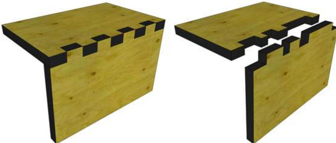
This arrangement of interlocking tabs and slots at a ninety degree angle is, of course, ancient and rudimentary. Most people call it a "box joint." It, too, can be biased by breaking symmetry.
