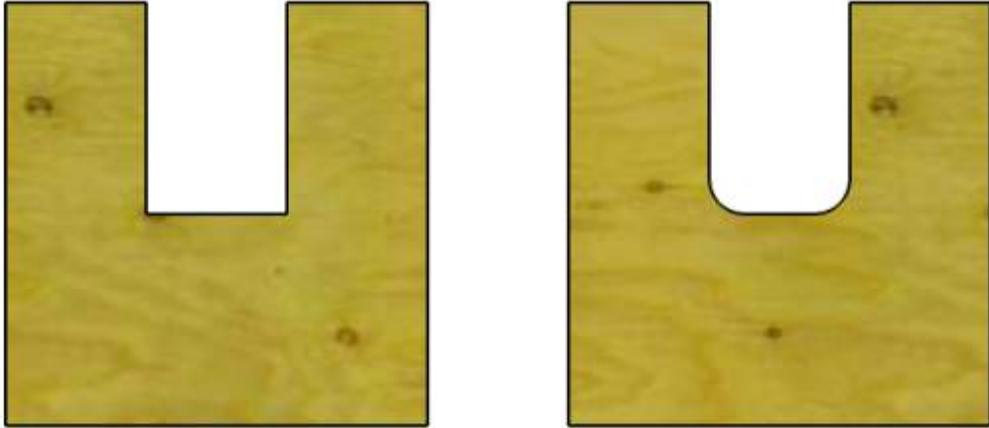
The laser-cut version, with its sharp 90 corners, is suitable for use in a simple edge-lap joint:
