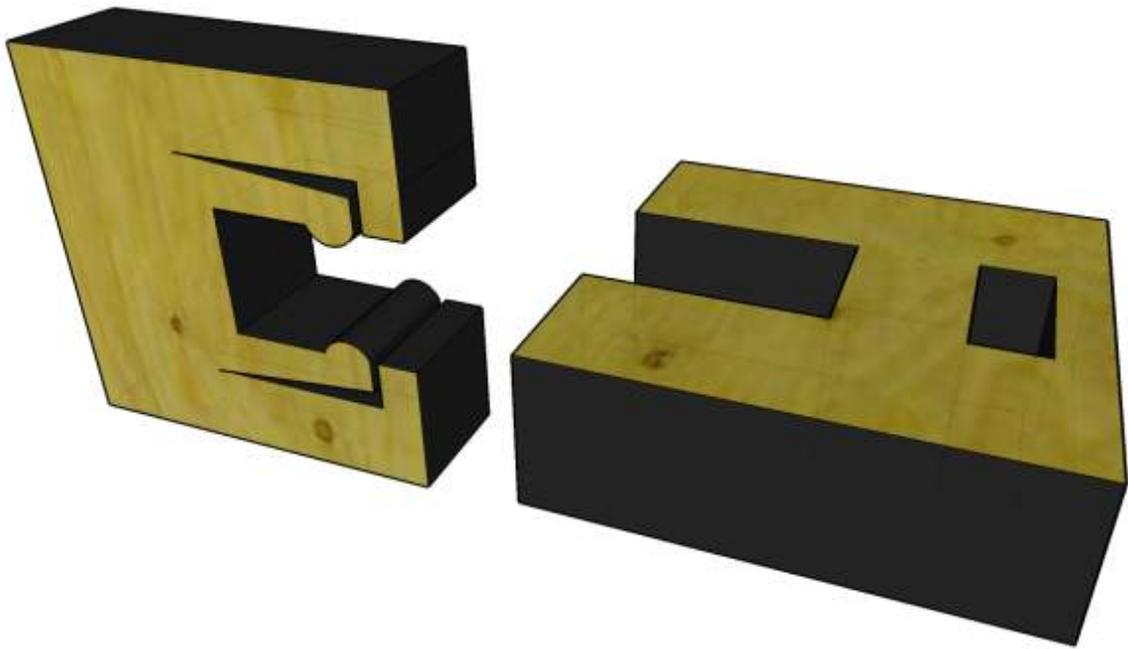
Replace the hook with a bulge and the snap becomes a detent: The part will "stick" in place but can be removed with sufficient force.
