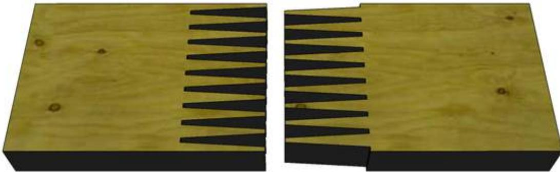
Here, for instance, is the classic "finger" joint, used to join members in the same plane for gluing.
