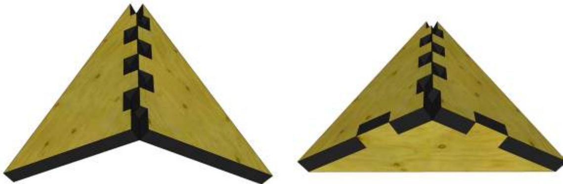
The bottoms of the slots no longer index closely against the surface of the stock, but if the members are held in alignment by some other means, for example by glue or the introduction of a third panel (as shown to right), it may not matter.
