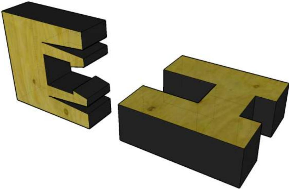
Here's a version of the basic slotted "edge lap" joint in which one side has an integral snap-lock feature. The snap hooks are accessible from the end of the joint. Insert a small flat-blade screwdriver, pry a bit, and they can be popped loose and the joint opened again.
