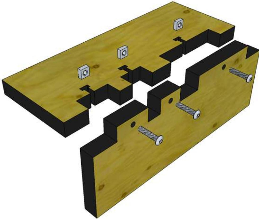
And it is just as amenable to the bolted captive-nut arrangement.
