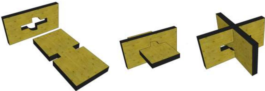
Here's a more unusual "X" joint that uses a radial interlocking motion to seal the deal.
