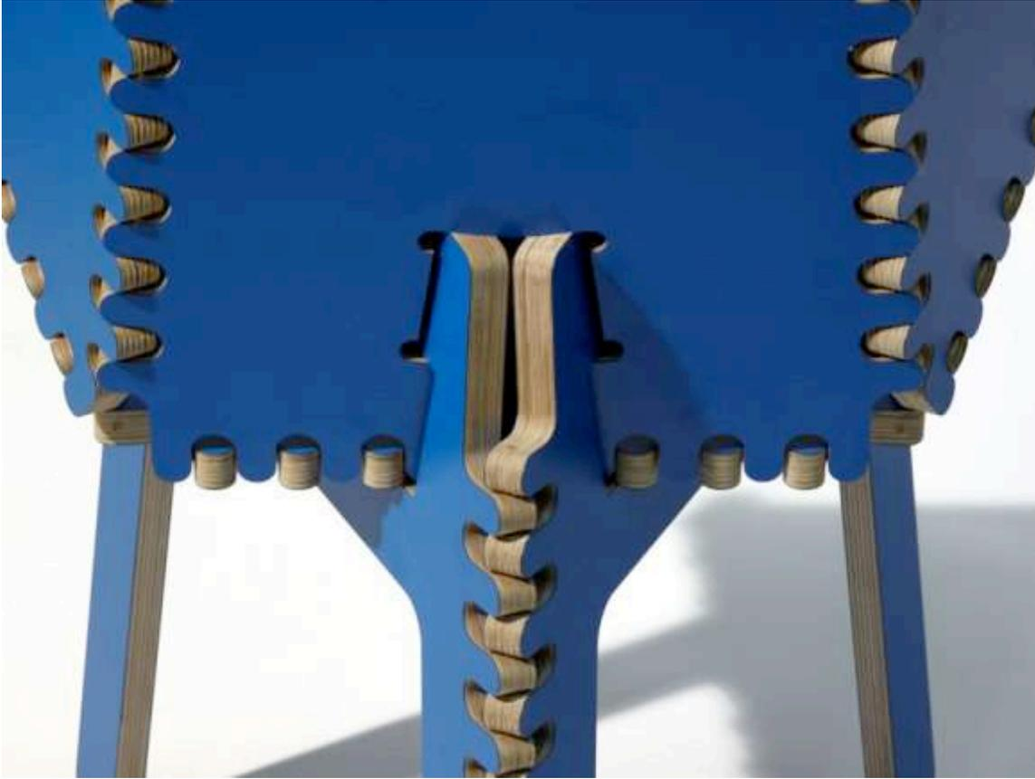
Sebastien is using pins, I believe, running longways through both sets of fingers, along the axis of each joint, which requires an out-of-plane drilling operation that is technically disallowed under our rules. But these joints could certainly be glued. If using glue, however, the rounded fingers, through they may look better, will limit the surface area available to the adhesive.
