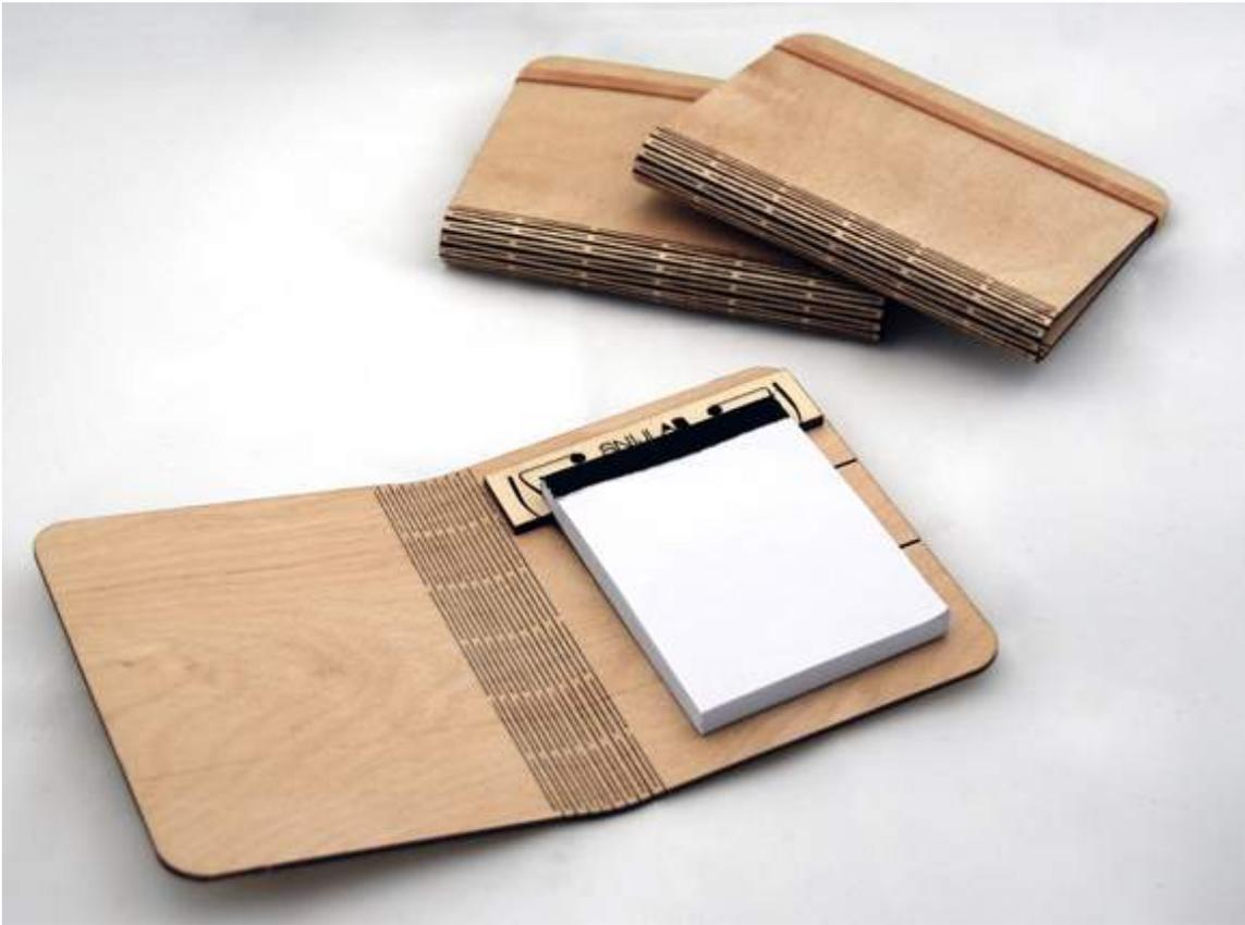
This is the somewhat famous Snijlab living hinge technique (which I continue to believe should be called a "sninge"), an accordion-cut pattern that allows for stable out-of-plane flexing. It is most commonly executed in laser-cut plywood, but there's no reason it couldn't be cut with a CNC mill and/or in other materials, though a router-cut sninge will have to be longer to achieve the same degree of flexibility as a laser-cut version, because the router slots will have to be considerably wider.
