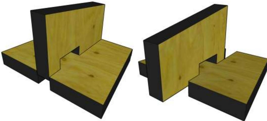
Often it is possible to deliberately break this symmetry so that the parts can only be assembled in one way, or at least in fewer or more obviously correct ways. Now the joint can still be assembled incorrectly, but the disfavored orientations are more obviously wrong, because the part edges no longer align.
