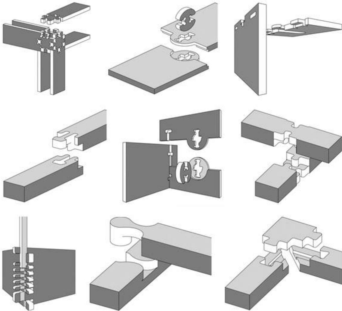
For this article, though, I'm deliberately considering a very limited case: Two (or even just one) cut parts, no partial-depth cuts, and a cutting axis always at 90 degrees to the surface of the stock. Even with these limitations, the possibilities are rich.
