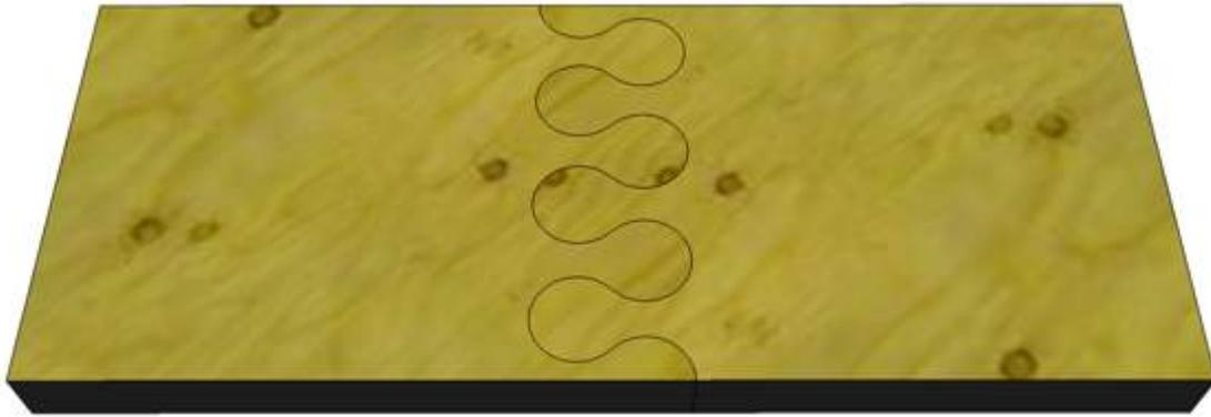
This interlocking "bulbed" version doesn't depend on glue for its strength in tension. If left unglued, of course, these flat joints require some means to keep the two pieces in the same plane when the joint is in use. Here is a variation of the "bulb" joint that allows for in-plane hinging action:
