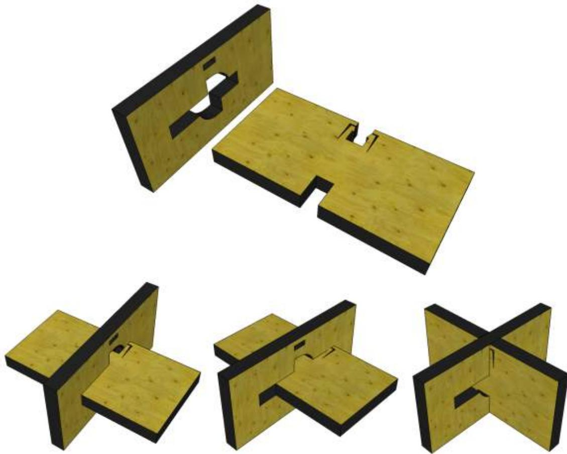
...and/or to the rotated member, as shown here. Note, in this case, that it doesn't matter if the profile of the catch is hooked or rounded: Once the catch pops into the slot, it'll be very hard to get out. For the reversible version, move the slot and the catch out to the edge of the stock.
