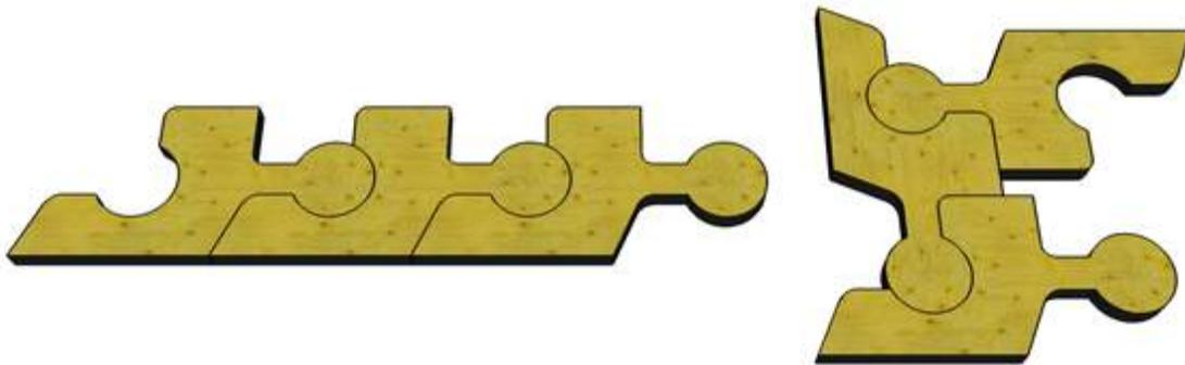
Kanelba hinges can be daisy-chained to make "snakes." The individual hinges, of course, can be set to "stop" at angles other than 90°.
