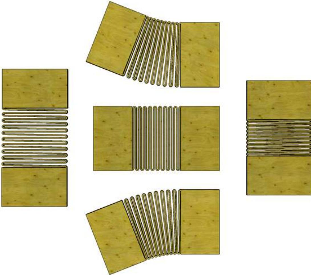
This is an in-plane spring or living hinge element that is kind of like kerf-bending, but with "thru" cuts. If not constrained to motion in the plane, such a feature will be pretty unstable. Here's a version more suitable for out-of-plane bending:
