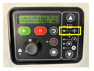
Push the joystick up or down to move the bed until material touches the focus tool. The laser is focused when the material and the focus tool are touching. Put the tool back once you're done
